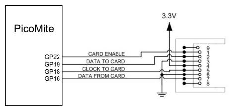
Note that you can use many different configurations using various pin allocations – this is just an example based on the configuration commands listed above.
