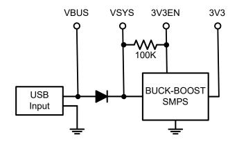
For embedded controller applications generally an external power source (other than USB) is required and this can be connected to VSYS via a Schottky diode. This will allow the PicoMite to be powered by whichever supply is producing the highest voltage (USB or VSYS). The diodes will prevent feedback into the lower voltage supply.
