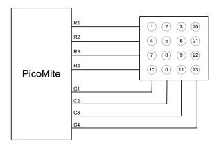
The detection and decoding of key presses is done in the background and the program will continue after this command without interruption. When a key press is detected the value of the variable var will be set to the number representing the key (this is the number inside the circles in the diagram above). Then the interrupt will be called.
