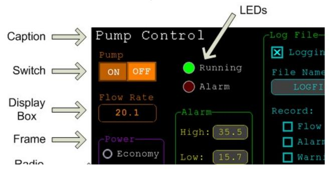
Each control has a reference number called '#ref' in the description of the control. This can be any number between 1 and the upper limit set by the OPTION CONTROL command. This reference number is used to identify a control. For example, a check box can be created with a reference number of #10:
