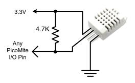
To get the temperature or humidity you use the HUMID command with three arguments as follows: BITBANG HUMID pin, tVar, hVar [, DHT11]
