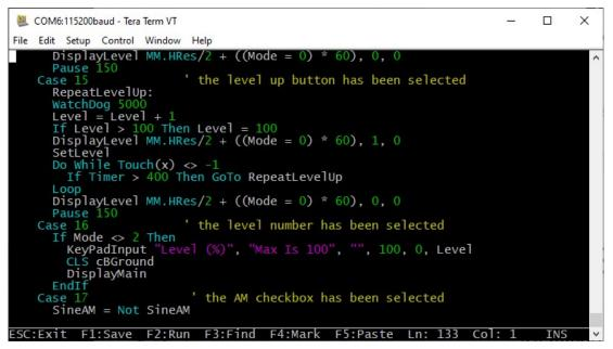
When the editor starts up the cursor will be automatically positioned at the last place that you were editing or, if your program had just been stopped by an error, the cursor will be positioned at the line that caused the error. At the bottom of the screen the status line lists details such as the current cursor position and the common functions supported by the editor.
